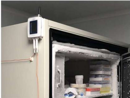
ULT Freezer (Cobalt X / PT100 Sensor)
