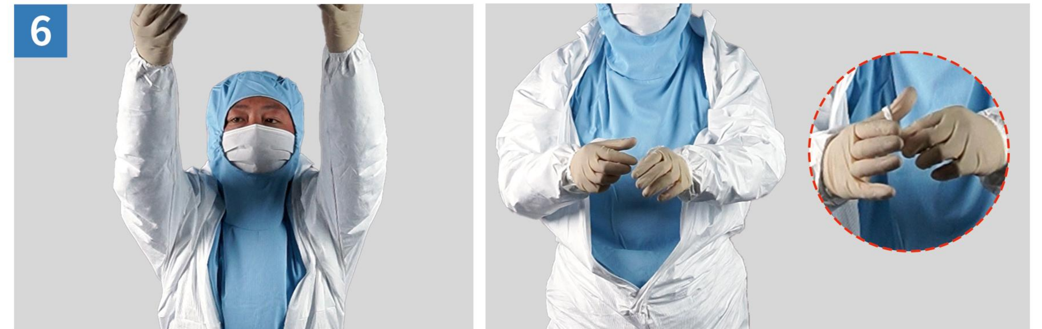
6 Insert your arms into the sleeves, leaving your hands exposed, and put the loops on your thumbs.
