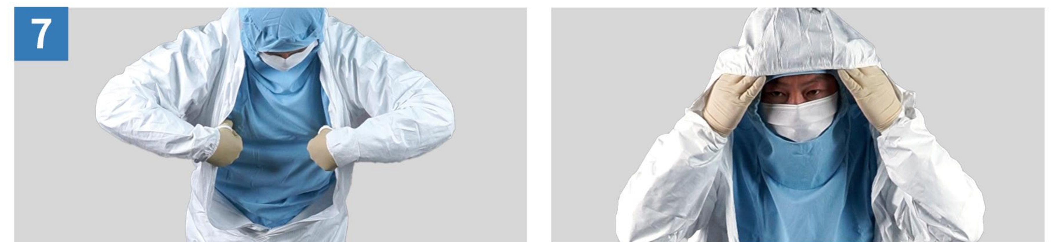
7 Gently bend over, insert your hands into the inside of the cleanroom coverall, trace upwards to the position of the hood, and put on the hood.
